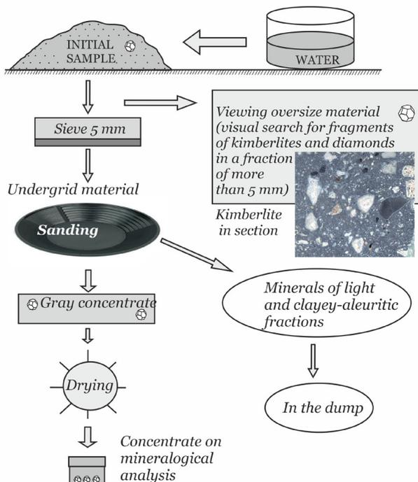
Fig. 24. The scheme of small-volume concentration of sand-gravel-pebble deposits on a shaker, used by the author in the field.
