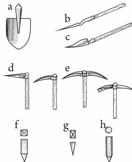
Fig. 17. Tools for driving mine workings manually (according to A. R. Sushon, 1976): shovels: a - spade, b - tunneling, c - loading (scoop); picks: d - one-sided (straight and oblique), e - double-sided; wedges: f - square, g - rectangular, and h - round.
