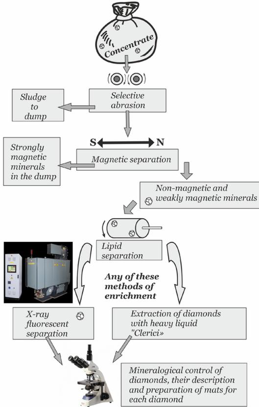
Fig. 27. Principal diagram of the extraction of diamonds from the field concentrate.
