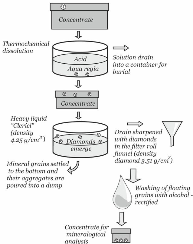
Fig. 25. Scheme of laboratory analysis of diamond concentrate.
