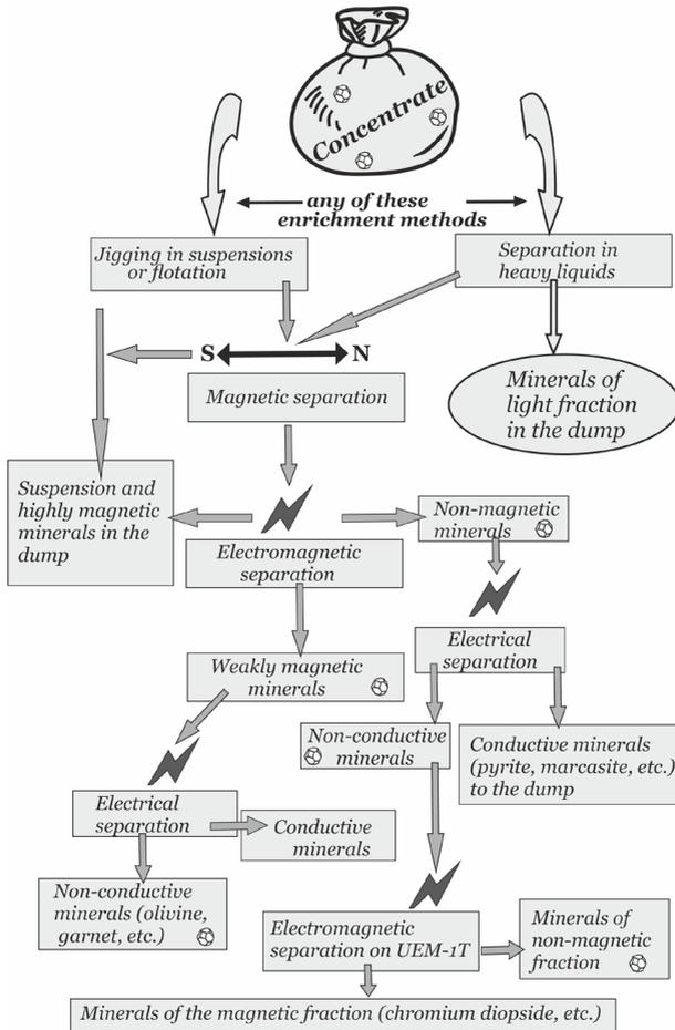
Fig. 26. Diagram of the sequence of extraction of heavy diamond concentrates (HDC) from placer concentrate.
