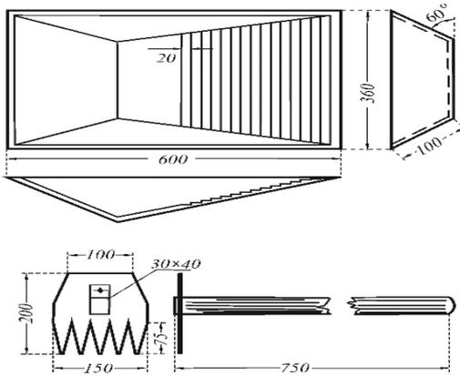
Fig. 19. Prospector tray with grooves on the flush plane and a paddle for removing coarse-fragmented material, and crushing clay pellets during screening.
