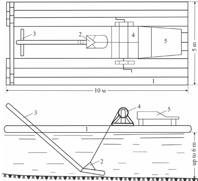
Fig. 35. A raft for sampling channel sediments (according to V. M. Kreiter, 1940): 1 - log raft, 2 - iron scoop, 3 - scoop handle, 4 - hand crank, 5 - cradle.
