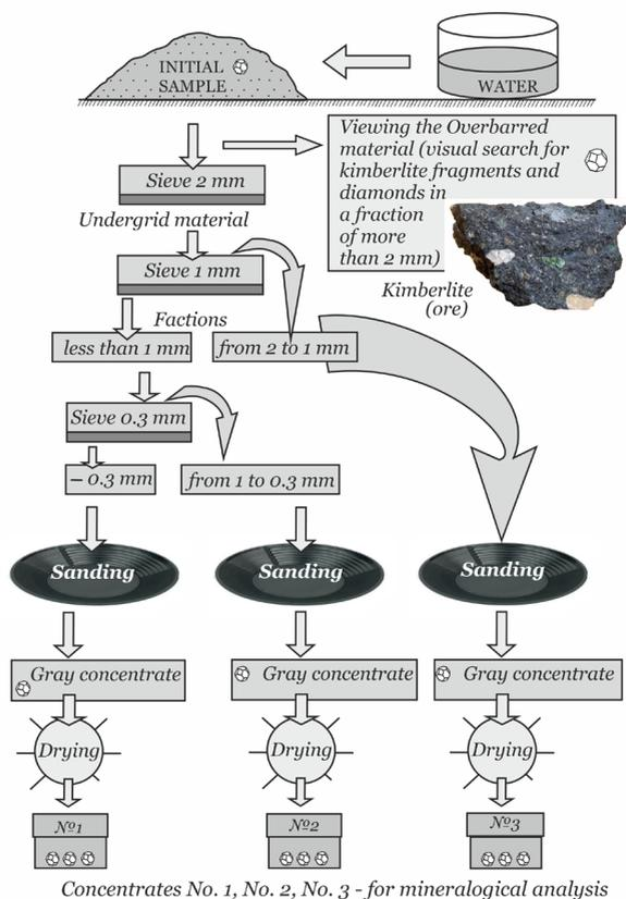
Fig. 23. Elementary enrichment scheme by obtaining a concentrate from the investigated loose deposits in a placer tray.
