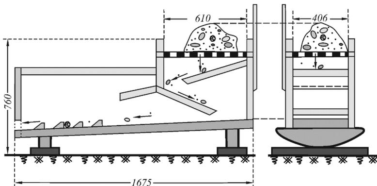
Fig. 22. American rocker (dimensions are given in millimeters) (after V. M. Kreiter, 1940).
