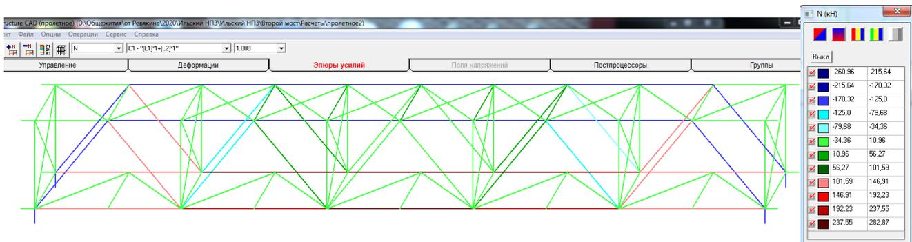
Fig. 3. N forces in elements obtained in StructureCad PC
