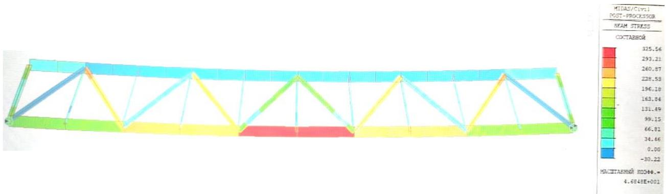
Fig. 3. N forces in elements obtained in the Midas Civil PC
