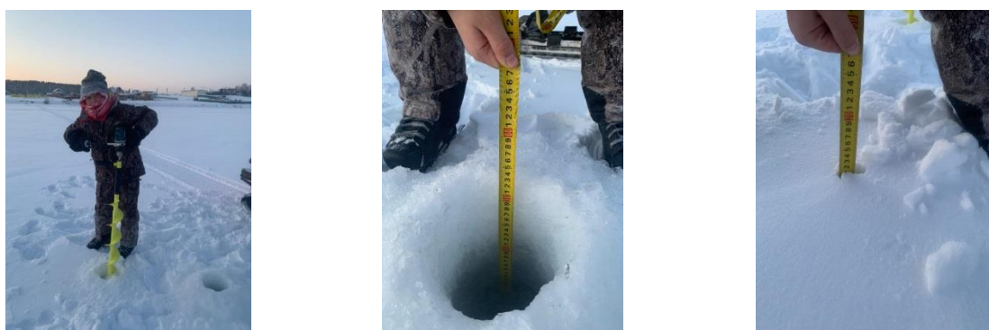
a) preparation of the hole b) measuring ice thickness c) measuring the thickness of the snow cover
