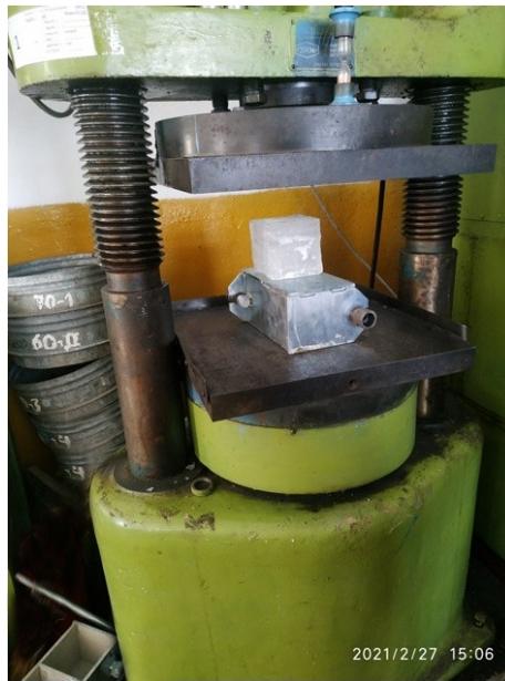
Fig. 5. Test of ice cubes for strength
