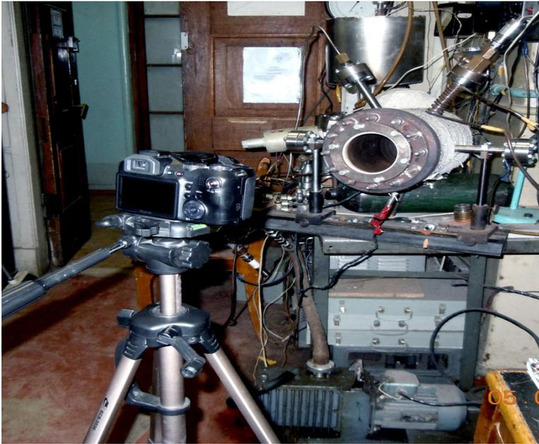
*Figure 2. The location of the high-speed video camera for filming the combustion process*
