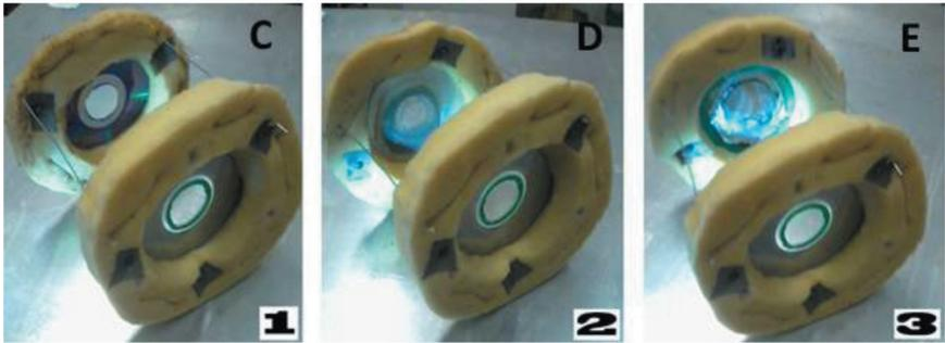
**Figure 5.** Complex obstacles, consisting of a flat obstacle with a diameter of 14 cm with a single hole 25 mm in diameter and a second flat obstacle with a single hole of 25 mm in diameter (1), a second flat obstacle with a single hole 25 mm in diameter, covered with a flat mesh (2) and a second a flat obstacle with a single hole 40 mm in diameter, into which a mesh sphere was inserted (3)
