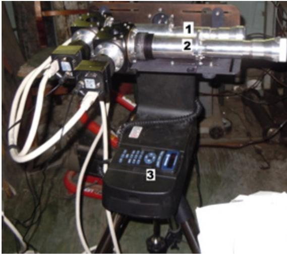
*Figure 15. Assembly of two hyperspectrometers VID-IK3 and VID-IK3 modified on a rotary scanning device*
