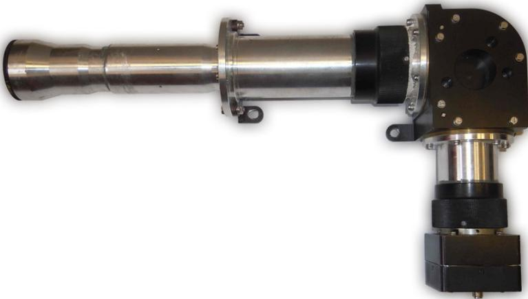
*Figure 4. Photo of a VID-IK3 hyperspectrometer*
