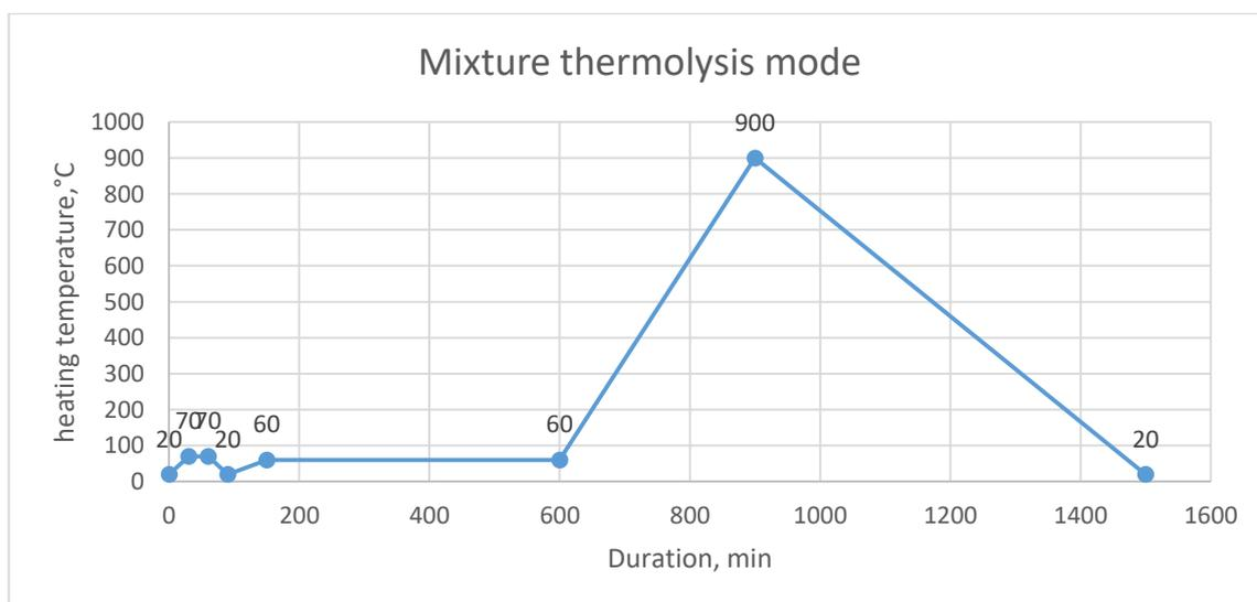
Figure 2. Graph of the heat treatment mode of the mixture
