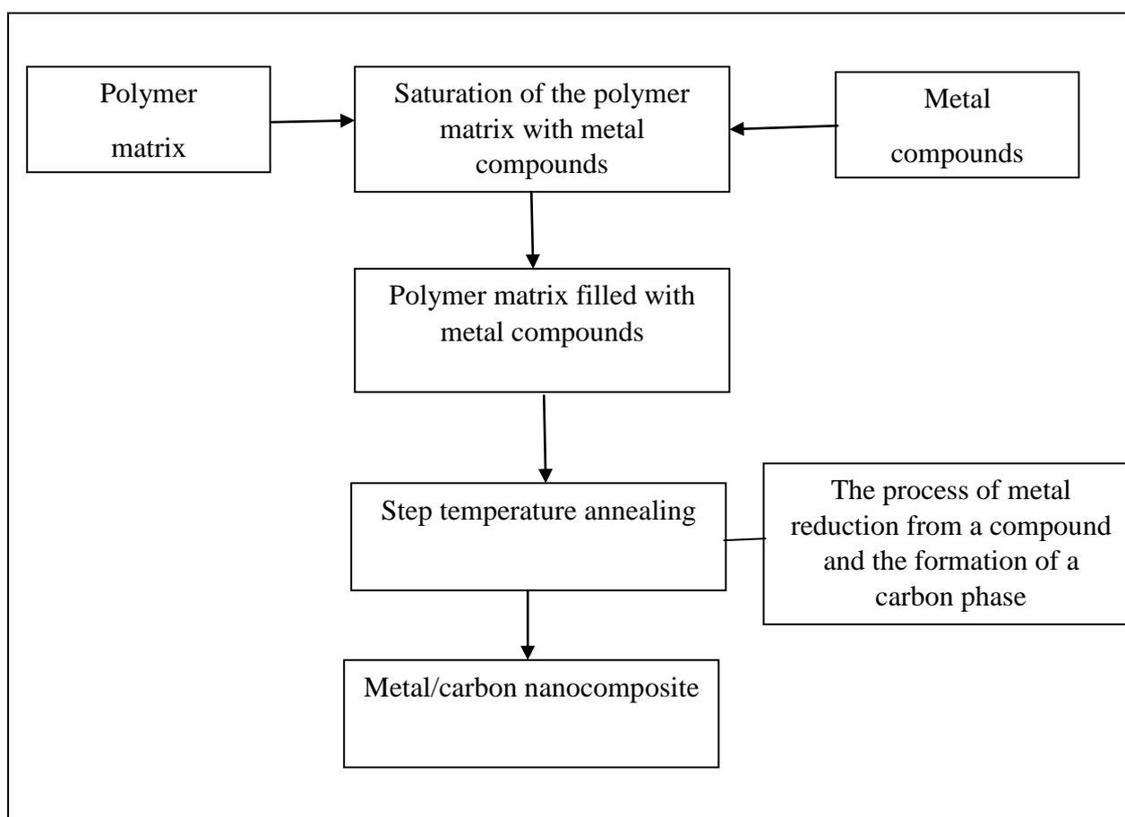
Figure 1. Scheme of obtaining metal-carbon nanocomposites
