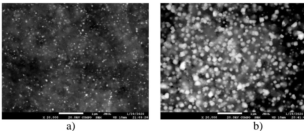
Figure 3. Morphology of Co/glassy carbon nanocomposite obtained using cobalt phthalate: a) in the upper part, b) in the lower part of the sample
